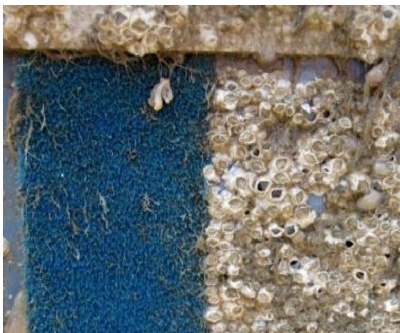
Figure 4. Antifouling activity of the barnacle encapsulated CuONPs.
