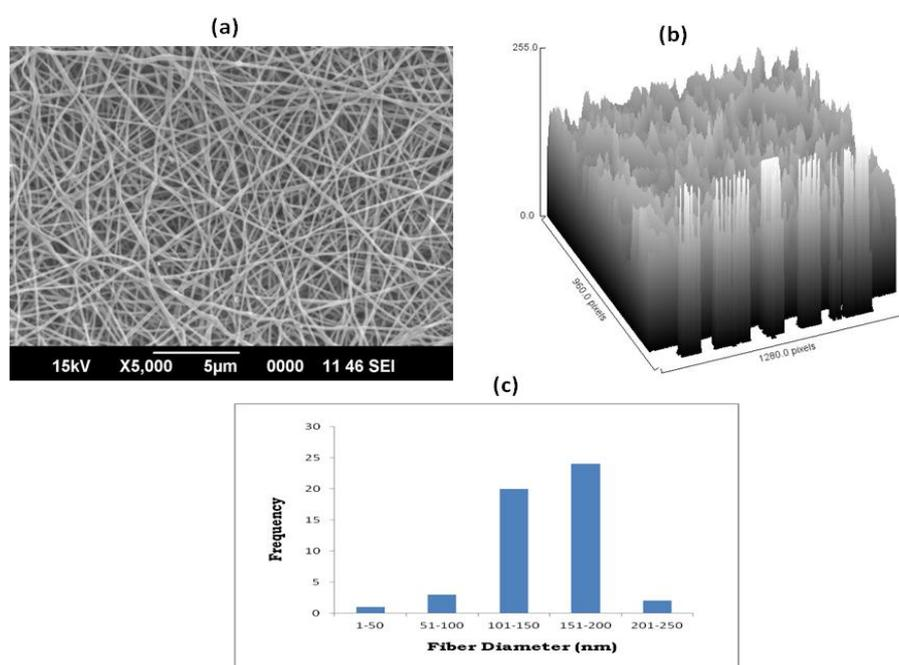
**Figure 3:** SEM micrograph (b) Three dimensional surface plot and (c) Fiber diameter distribution graph of PVA/MMT nanofiber mat
