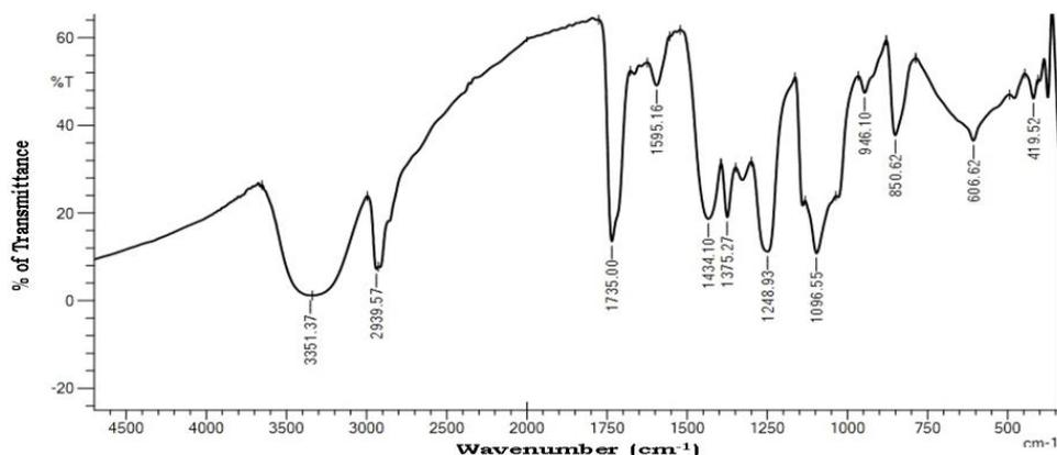
**Figure 1:** FT-IR spectrum of Polyvinyl alcohol/Montmorillonite clay nanofiber mat
