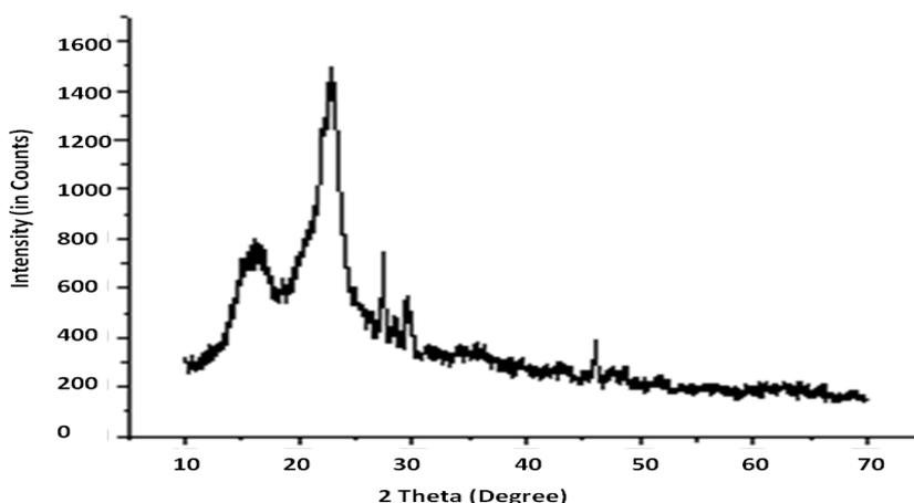
**Figure 2:** XRD pattern of PVA/MMT nanofiber mat
