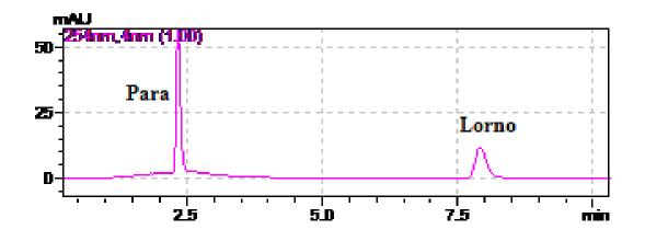
ANALYSIS OF FORMULATION: Preparation of standard solution: 100 mg of Paracetamol and 1.6 mg of Lornoxicam diluted with the Mobile phase up to 100 ml (Stock Solution).
