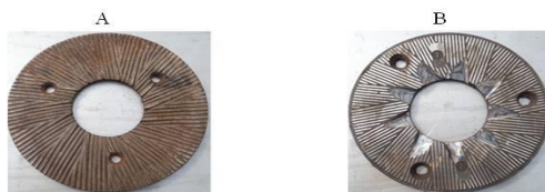
Figure 2: Grinding discs (a) new, (b) worn {used} for locally fabricated grinding machine (see Fig 1.C)
