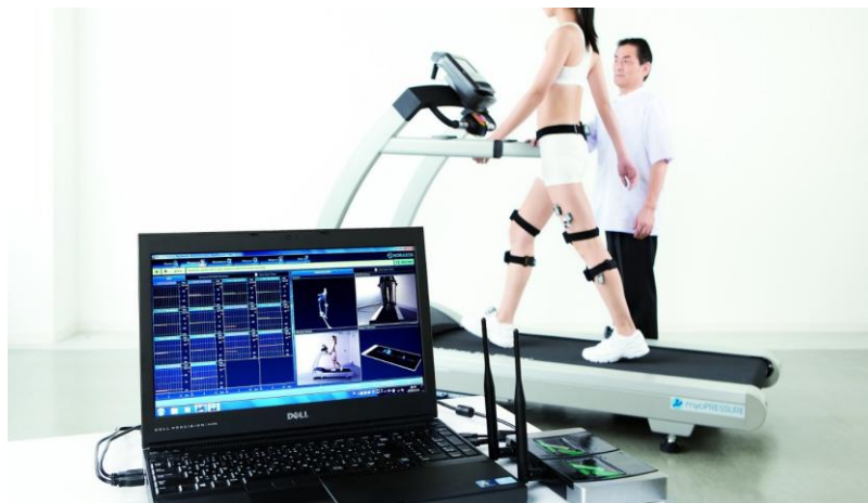
Figure 1- Noraxon pressure mat treadmill used for impact forces and muscle activity.
