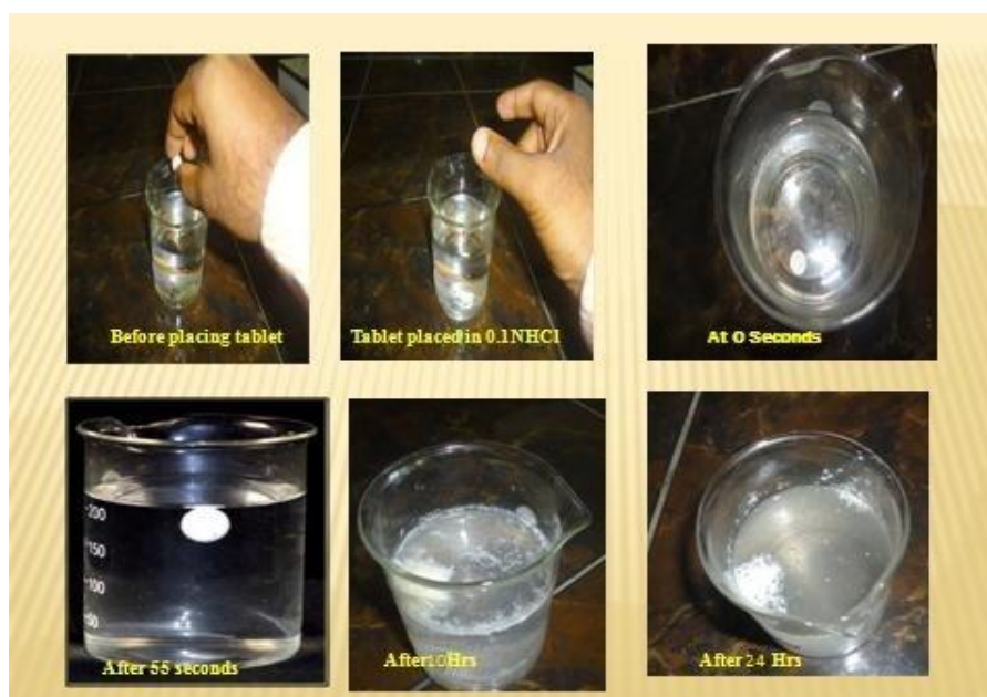
Fig.No.37. Imagetaken during invitro buoyancy study of formula F10 in 200mL 0.1N HCl at particular time intervals.
