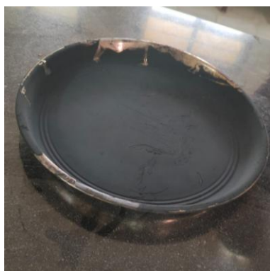
Fig 13: Black soot deposited on steel plate
